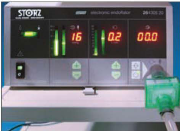
Fig. 11 The intraabdominal insuflation pressure shown on the front panel of the ELECTRONIC ENDOFLATOR® is inappropriate .
